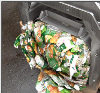
Figure: Volume of Tetra Pak® at the outlet
